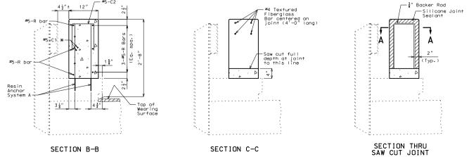
Guidance: Remove top slopes from ends in Elevation for 2'-8" blockout. Alternate details for 2'-8" blockout
