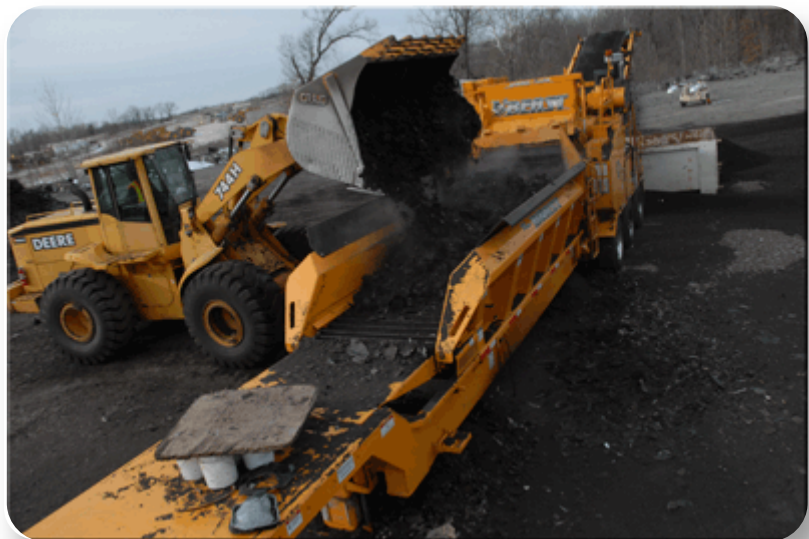
Shingles are ground up and processed
