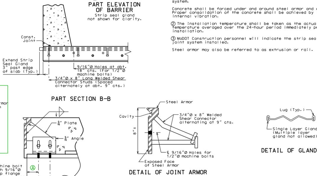
**Table of Allowed Transverse Strip Seal Expansion Joint System**
