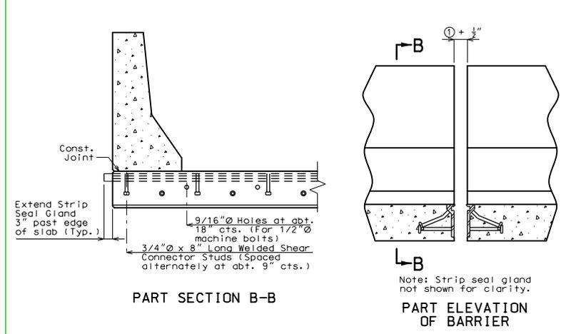
Alternate details for Type B barrier (SBC)
