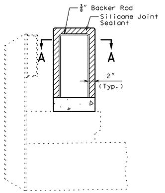
SECTION THRU SAW CUT JOINT
