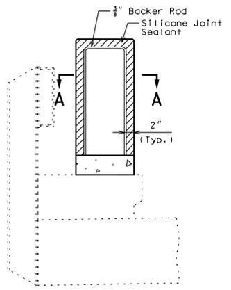
SECTION THRU SAW CUT JOINT
