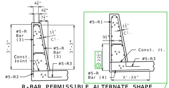
Use a minimum lap of 3'-1" for #5 horizontal barrier bars.
