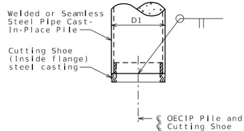
MANUFACTURED OPEN ENDED CUTTING SHOE (INSIDE FLANGE)
