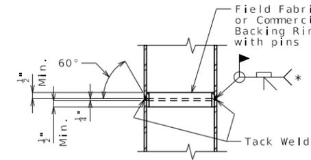
STEEL PIPE PILE SPLICE
