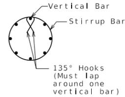
DETAIL OF SEISMIC (5) STIRRUP BAR
