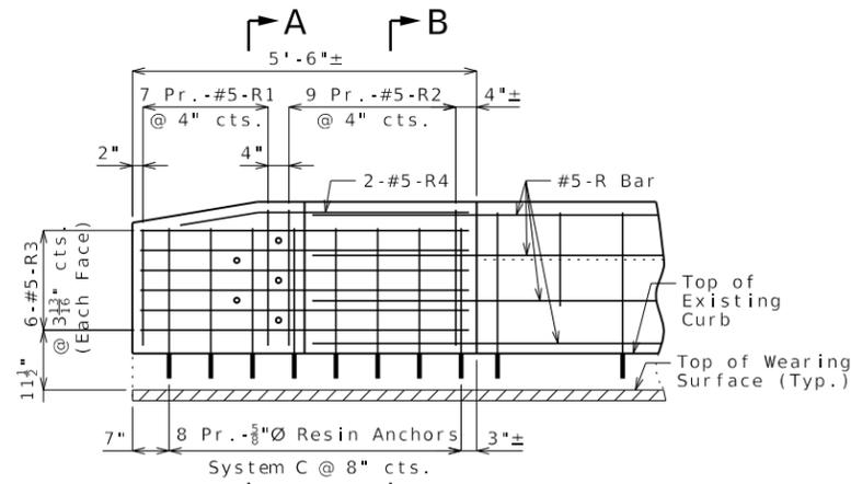
ELEVATION SHOWING REINFORCEMENT
